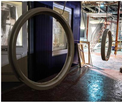
The circular window follows a very similar process where the aperture on-site is measured and our CAD technician draws both plan and section drawings that used by the CNC operator to cut the frame, sash, plant-ons and glazing bead. These items are then assembled in the joiners shop to ensure the tight tolerances account for painting. Both pivot hinges and finger pull latches are dry fitted and removed.
