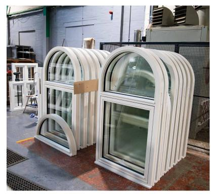
Engineered timber from Estonia is delivered into the 175,000 sq ft factory in Maryport, a small coastal town on the Solway coast of North West Cumbria. Here the timber is processed through a series of manufacturing processes that craft a modern high tech thermally efficient timber window ready for their installation into the historic Allerburn Manor in Alnwick, Northumberland.
